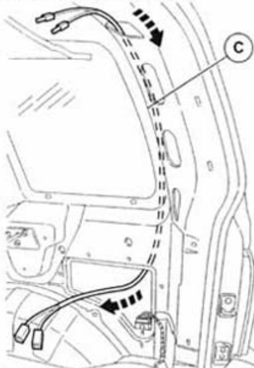
16 USED SUPPLIED CLIPS TO PROVIDE STRAIN RELIEF (4'-8" FROM CONNECTION POINTS).
